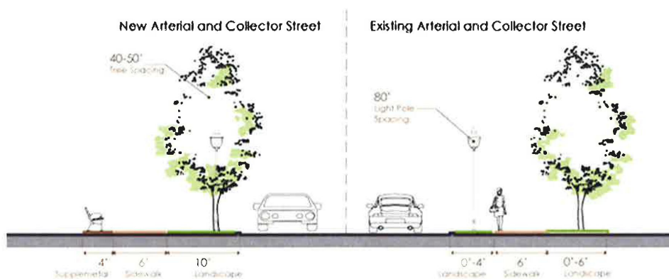
Streetscape Figure—Arterial and Collector Streets
